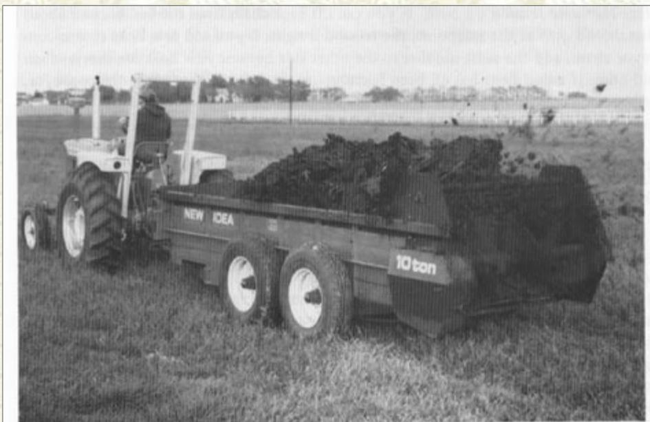
FIGURE 20-6. Showing the spreading action of the upper beater and lower widespread (Avco New Idea).
