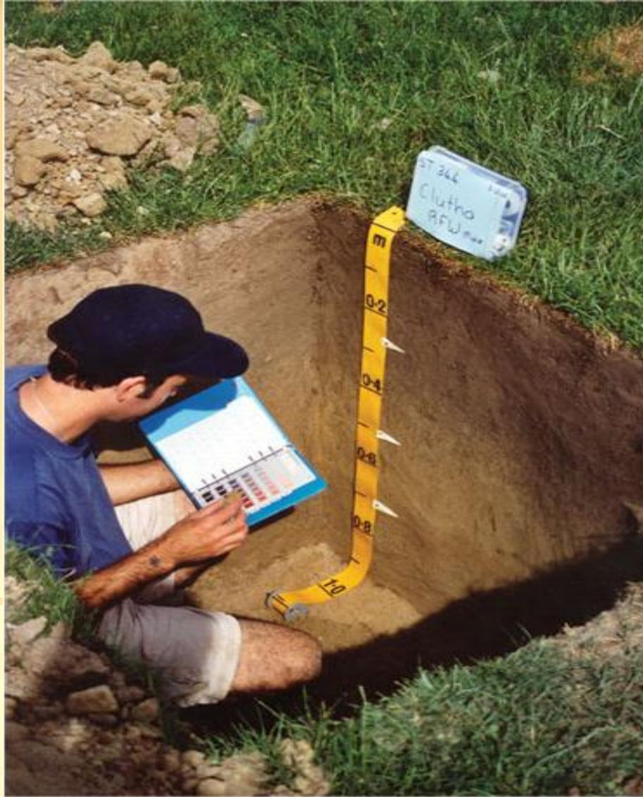
*Figure 1. The ultimate soil pit dug deep and wide to provide an excellent view of soil layers. The soil scientist is measuring soil colour using a soil colour chart.*
