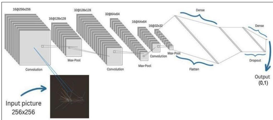
Fig. 4. CNN model Architecture.
