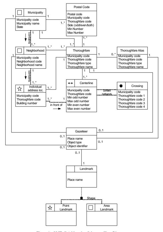
Figure 1 - OMT-G Addressing Schema - Class Diagram
