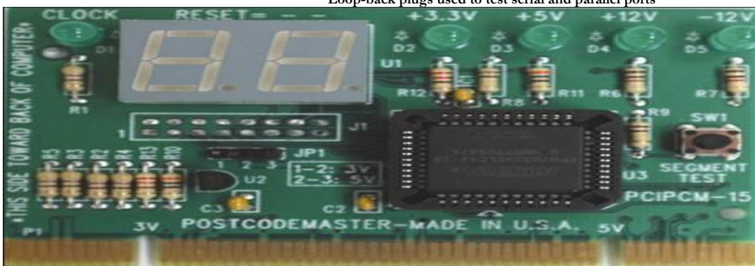
Post Code Master diagnostic card by MSD, Inc
