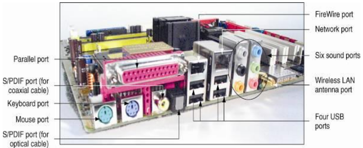
A motherboard provides ports for common I/O devices
