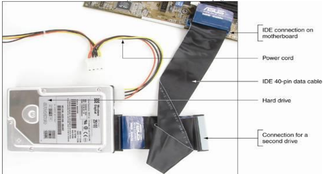
A PC's hard drive subsystem using parallel ATA
