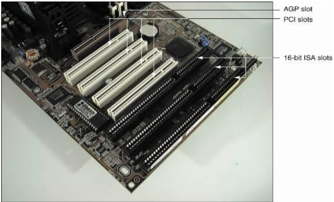
PCI bus expansion slots are shorter than ISA slots and offset farther; the one AGP slot is set farther from the edge of the board
