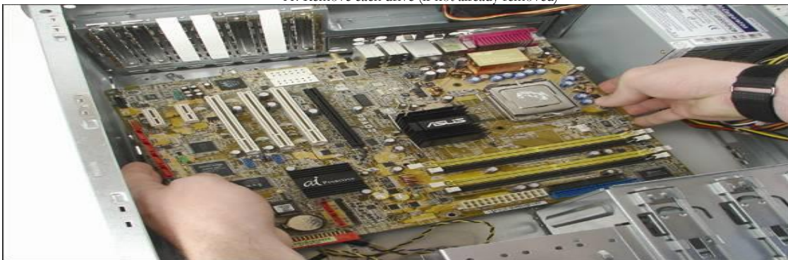
Remove the motherboard from the case
