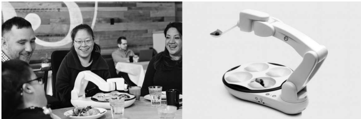
Figure 5.2 The Obi feeding robot. Obi is a robotic feeding device for those with upper extremity limitations. Obi allows its users to choose what they eat and control the pace of their meal. Obi increases independence, social inclusion, and enjoyment at mealtime ( www.MeetObi.com ).
