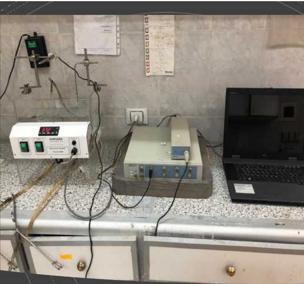
PowerLab (DAQ) Data Acquisition Hardware Device for Research
