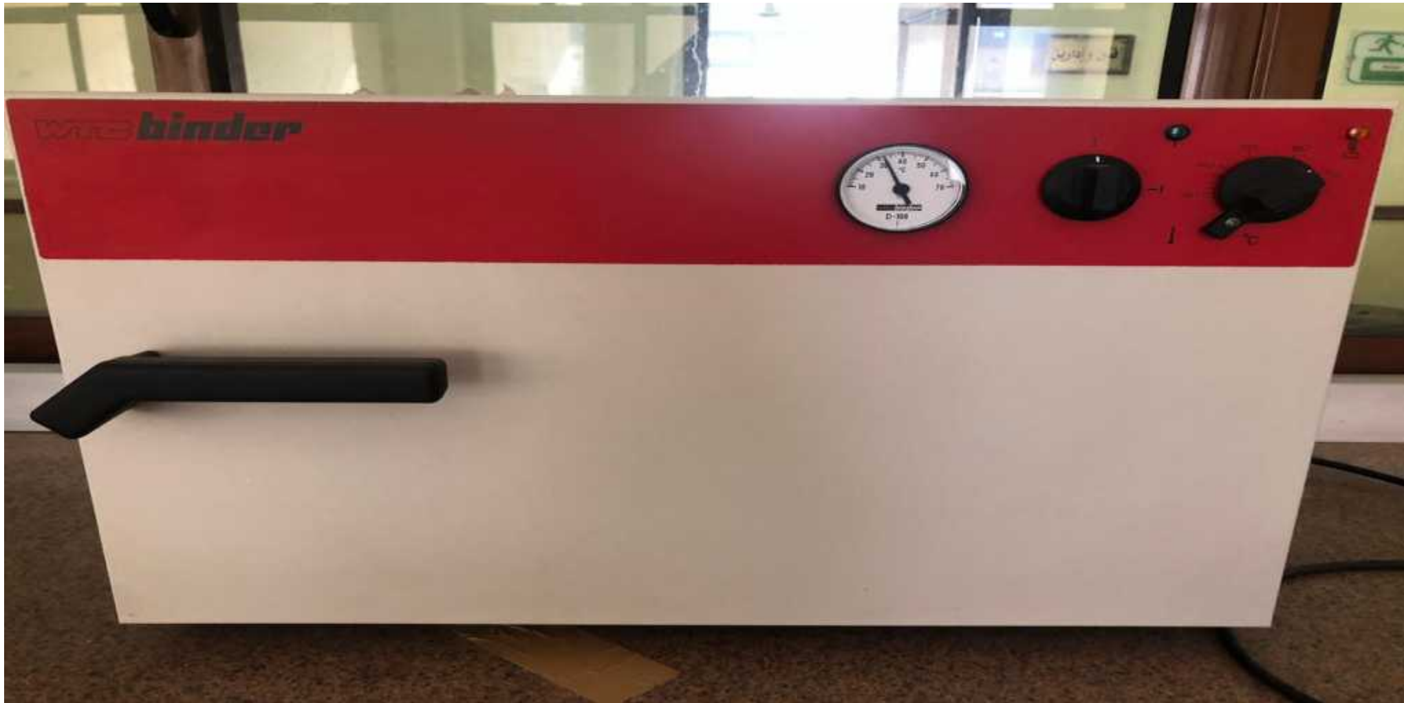
Incubators with mechanical adjustment for Drying and heating
