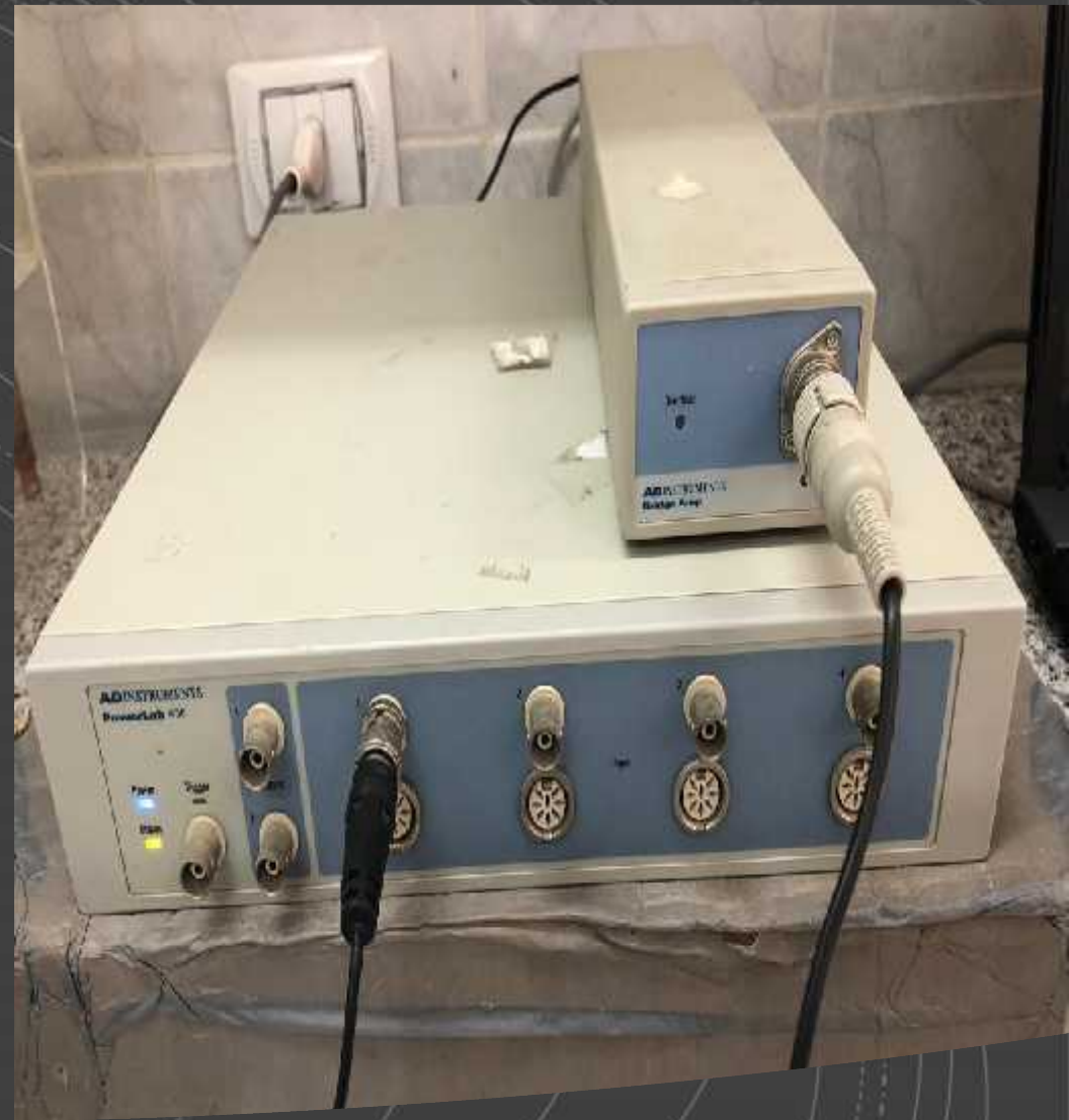
PowerLab (DAQ) Data Acquisition Hardware Device for Research
