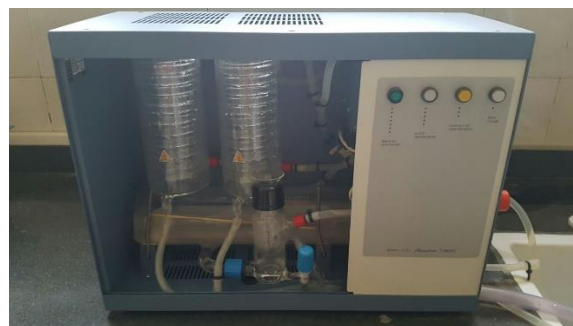
Water distillation system
